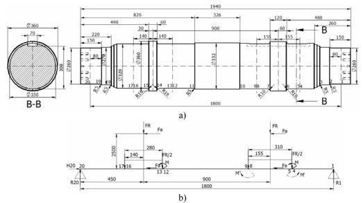
Fig. 3. Shaft design size and mathematical load model
