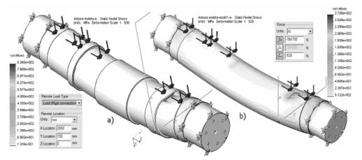
Fig. 7. Analysis with finite elements of the two shafts, existing and proposed
